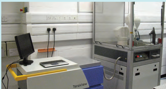
Figure 3. New THz imaging system, equipped with a robotic arm, at the Terahertz Research Group Lab
