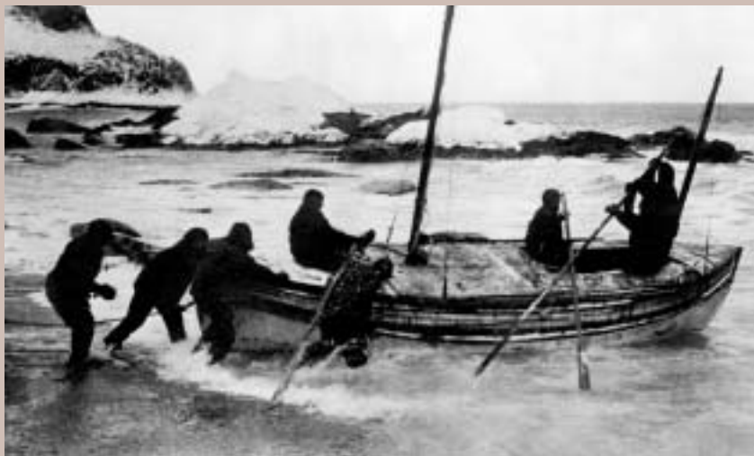
Launching the James Caird at Elephant Island, 24 April 1916. The Caird carried Shackleton and his five-man crew 800 miles to South Georgia in an epic seventeen-day voyage. Just 22ft long, with a 6ft beam, the boat was stabilised with 2000lbs of ballast to stop it capsizing. The decking was improvised from canvas and sledges
